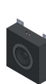
SA112N Type 2 way coax Power RMS/Max (W) 50/100 Loudspeaker (Ø cm) 13,0 Dim. (cm) 25,0 x 25,0 x 8,0 Impedance (Ω) 8
