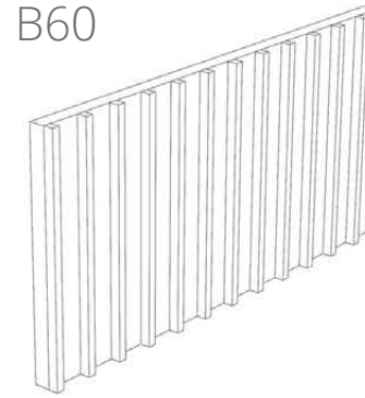
dimensions 60x120x7cm slat on the short side
