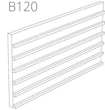
dimensions 60x120x7cm slat on the long side
